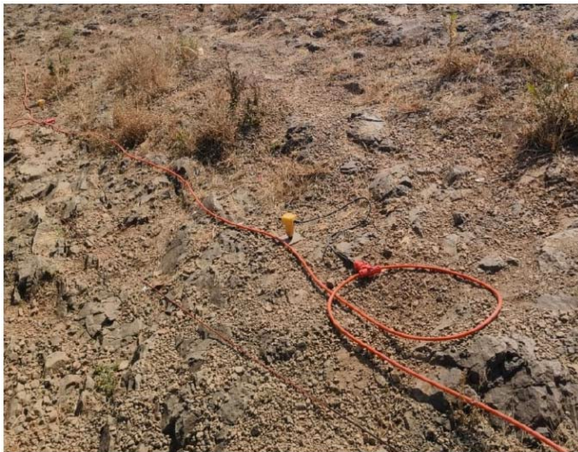
Figure 11: Geophone Array Arrangement for Surface Wave Data Acquisition.
