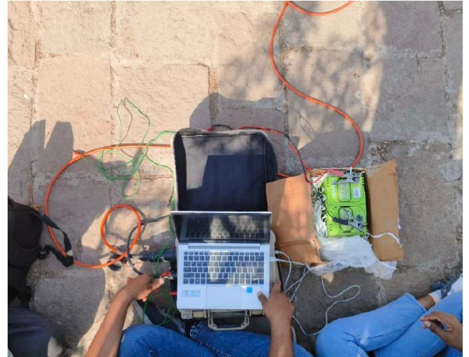
Figure 13: Portable Data Acquisition System with Power Supply and Control Unit.
