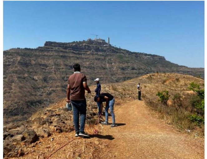
Figure 8: Preparation of MASW Survey Line at the Test Location.
