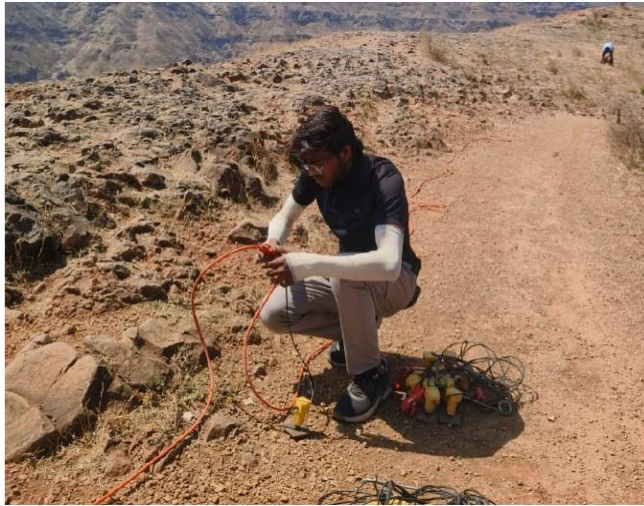
Figure 10: Installation and Connection of Geophones Along the Survey Line.
