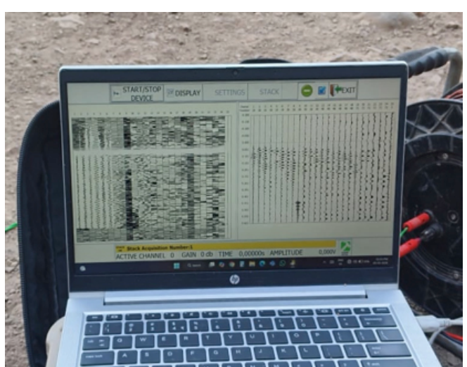
Figure 15: Display of Recorded Seismic Waveforms During Data Acquisition.
