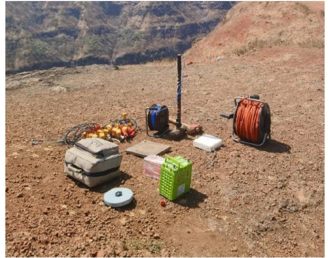
Figure 7: MASW Survey Equipment and Accessories Used for Field Testing.
