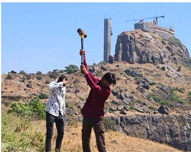
Figure 12: Generation of Seismic Waves Using a Sledgehammer Source.
